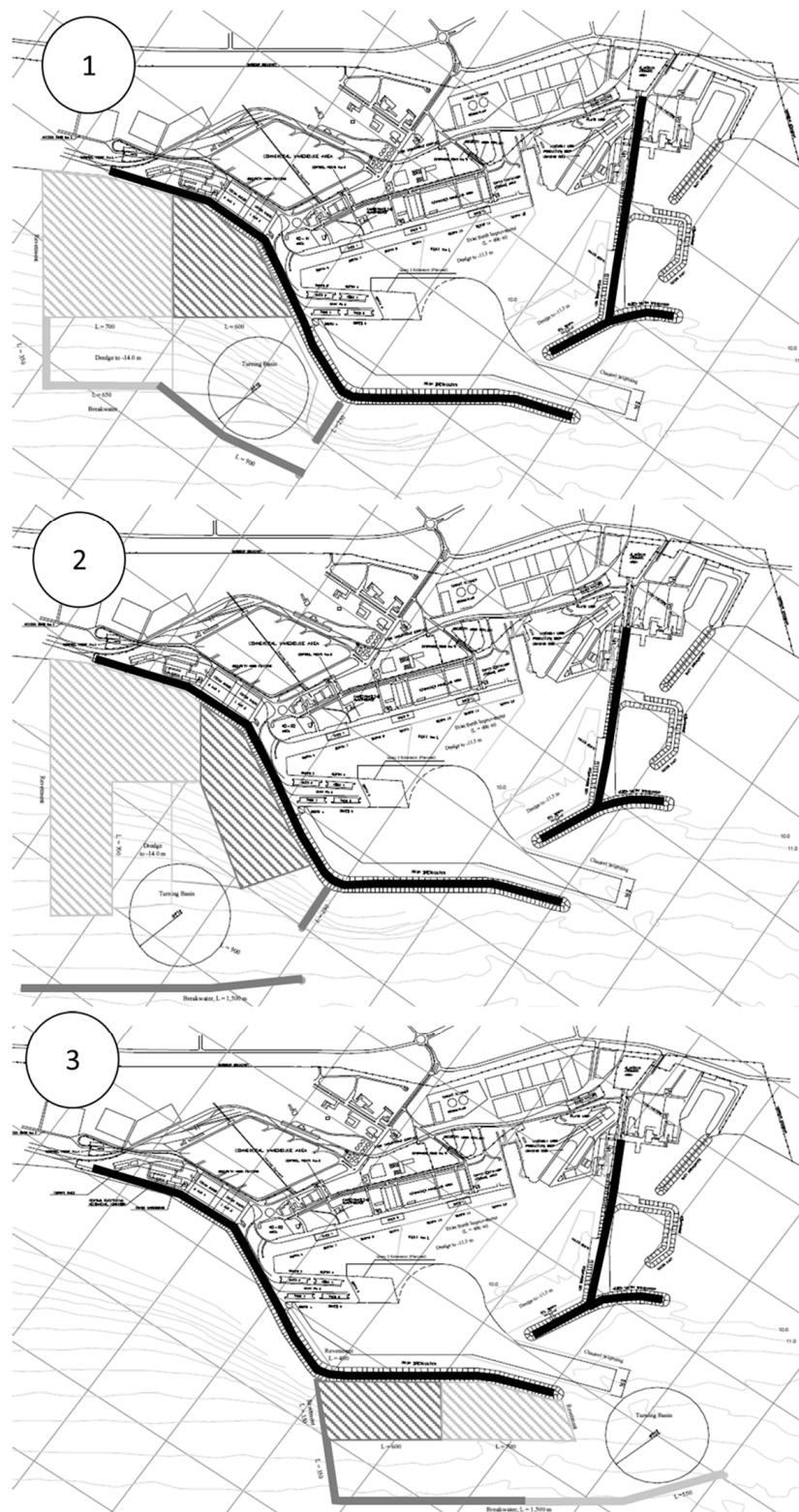
Figure 5. Port layout alternatives considered for Tema port expansion in the pre-feasibility study by JICA and GPHA; Alternative 1, 2, and 3 from top to bottom (adapted from [66]). In black, the breakwater layout before expansion; in dark grey, the first stage construction of the extended breakwaters (lines) and reclamation (diagonally shaded areas); and in light grey, the second stage construction of breakwaters (lines) and land reclamation (diagonally shaded areas).
