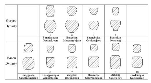
Figure 3. The Sections of cross-beams (source: author's edit [9]).
