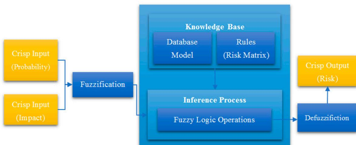
**Figure 1.** The structure of a fuzzy inference system, adapted from Urbina and Aoyama [17].
