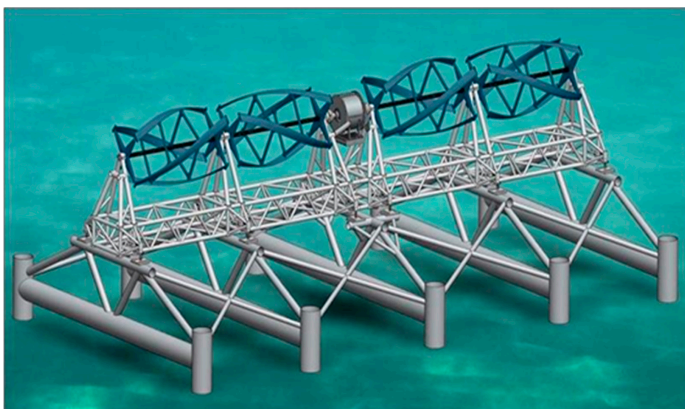
Figure 1. Illustration of Ocean Renewable Power Company’s TidGen® Power System with turbine and bottom support frame (length 31.2 m, width: 15.2 m, height 9.5 m).
