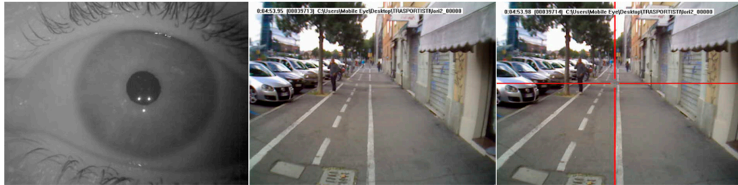
Figure 3. Superimposition of the eye tracking output to the cyclist's visual scene.
