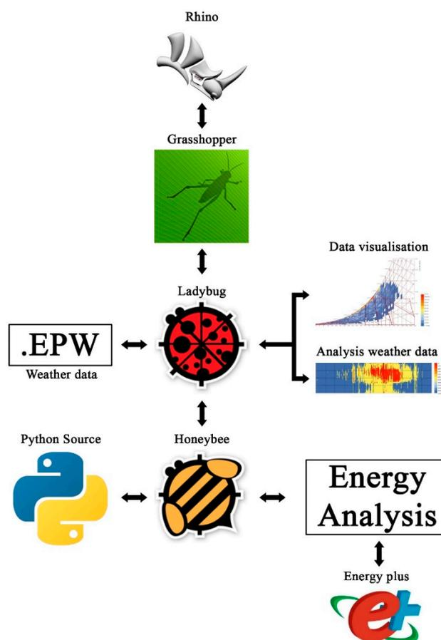
Figure 1. Linkage hierarchy of Rhino software plugins.
