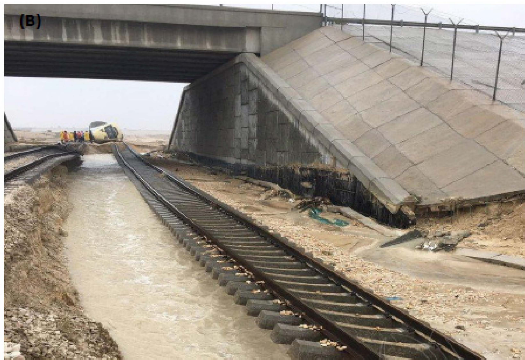
Figure 1. The Riyadh–Dammam train derailment. Image (A) shows the Riyadh–Dammam train derailment on 18 February 2017. Image (B) shows overturning of the Riyadh–Dammam train resulting from land drift due to floods.
