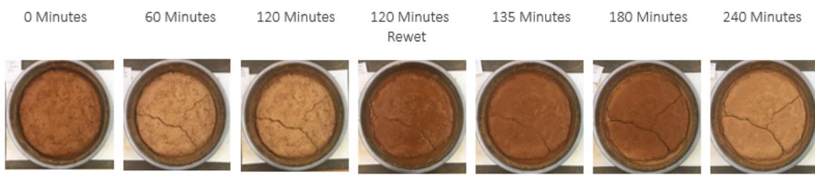
Figure 4. Desiccation crack test results for accelerated test for base soil.
