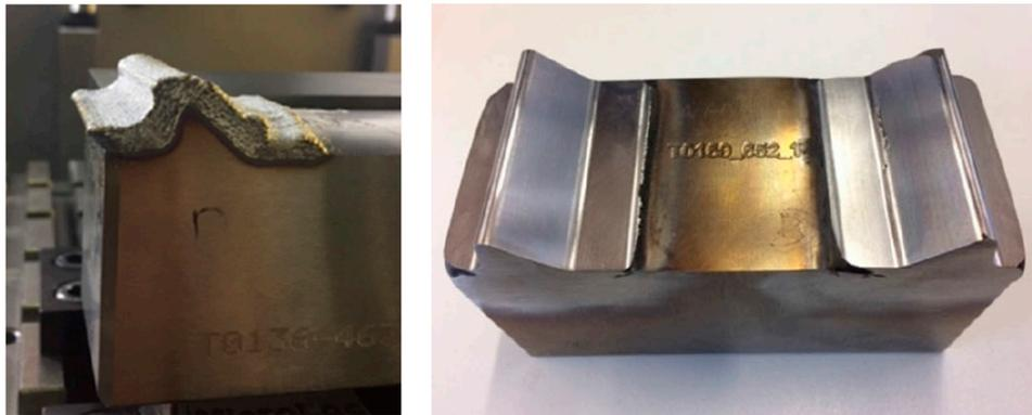
**Figure 7.** Mould repair using powder laser deposition before and after finishing [48].
