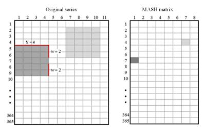
**Figure 1.** A scheme of the moving average over shifting horizon (MASH) process (Y = 4, w = 2,  $N_y = 11$ ) represents the number of years of the original time series, and  $N_h = 8$  represents the length of the resultant time series of MASH).
