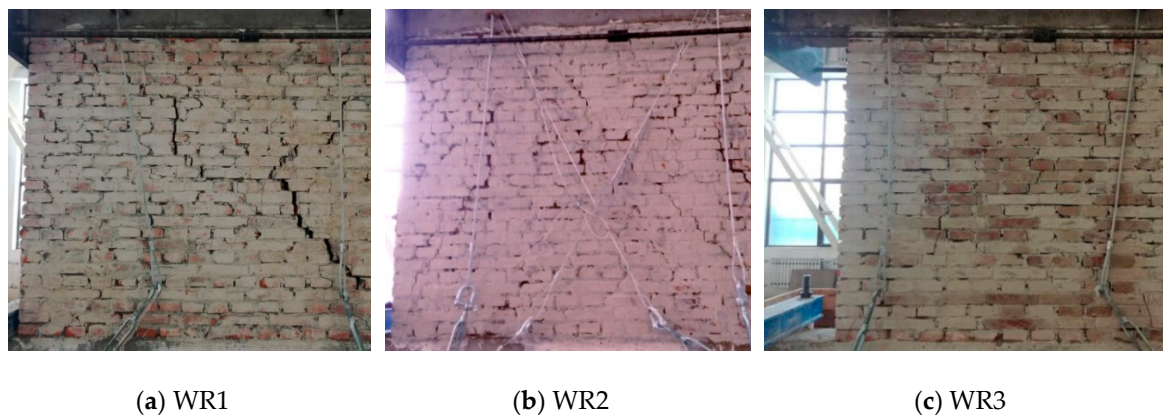
Figure 6. The crack distribution of un-reinforced masonry walls at the ending of tests.
