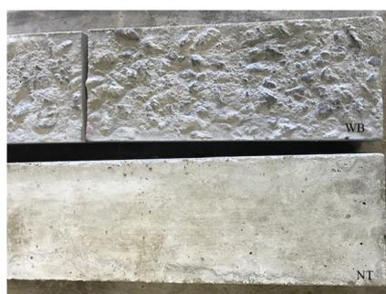
**Figure 2.** Substrate before and after surface treatment.
