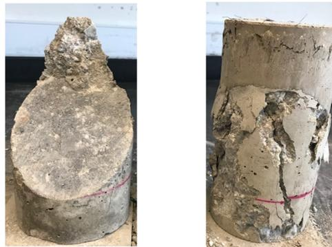
Type A: interface failure    Type B: substrate failure
