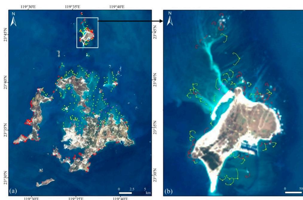
**Figure 6.** Spatial distribution of STWs (2018 Inventory) on the Penghu Archipelago (left) and Chipei Island (right). Red, yellow, and pink symbols represent arched, single, and double-room STWs, respectively. The base map consists of Landsat-8 OLI imagery that can be downloaded from <http://www.usgs.gov>.
