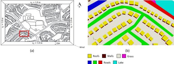
**Figure 5.** (a) Digital model of the study area, with computational boundaries and wind direction shown. (b) A close-up of the part of the study area highlighted in (a). H is the height of the buildings (5 m), while  $z_0$  is the aerodynamic aerodynamic roughness length of the parts of the model where the buildings were not explicitly resolved.
