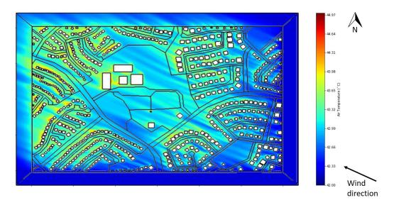
**Figure 8.** Air temperature at a 2 m height (in °C) for the Existing Pavements case with a far-field air temperature of 42.22 °C.
