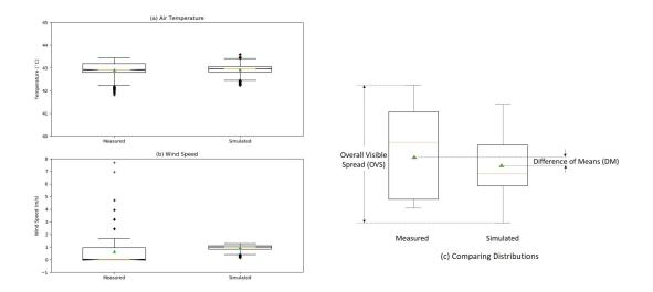
**Figure 7.** Box-plots of measured and simulated (**a**) air temperature and (**b**) wind speed at a 2 m height. The triangle in the middle of the boxes represents the mean value of the distribution. The definitions of Difference of Means (DM) and Overall Visible Spread (OVS) for comparing distributions are exemplified in (**c**).
