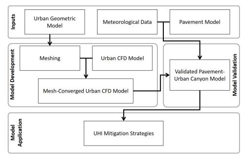
**Figure 4.** Flow diagram showing the steps towards development, validation, and application of the pavement-urban canyon model.
