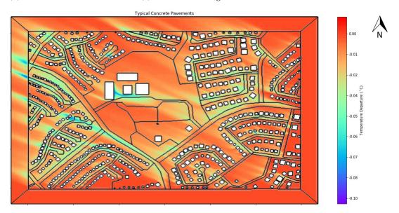
**Figure 10.** Difference of 2 m air temperature from existing conditions for the Typical Concrete Pavements scenario.
