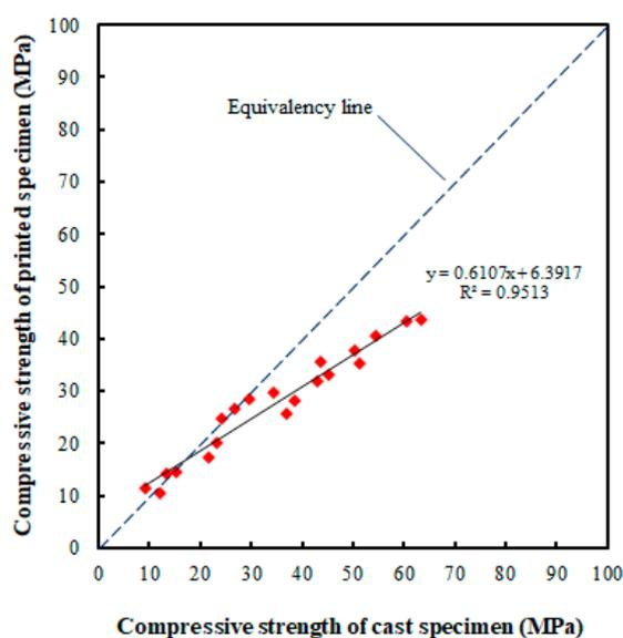
**Figure 7.** Relationship between cast and printed specimens' compressive strengths.
