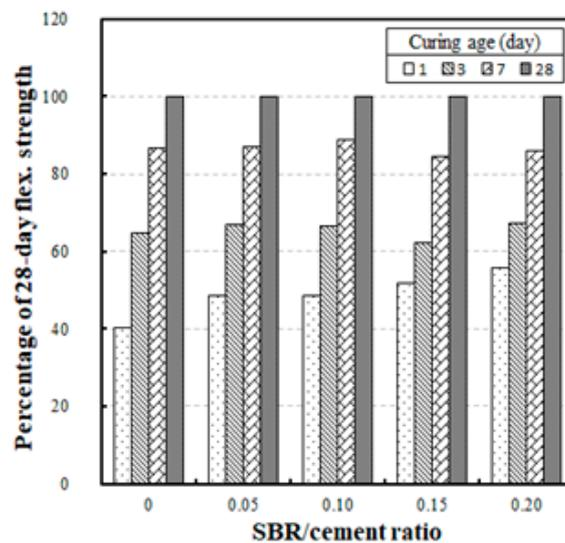
Figure 10. Relative gain in flexural strength and SBR/cement ratios for cast specimens with different curing ages.
