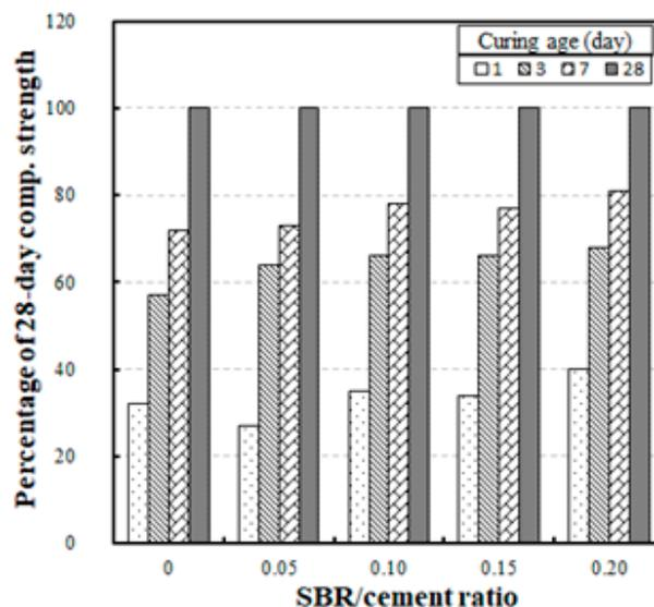
**Figure 6.** Relative gains in compressive strength and SBR/cement ratios for printed specimens with different curing ages.
