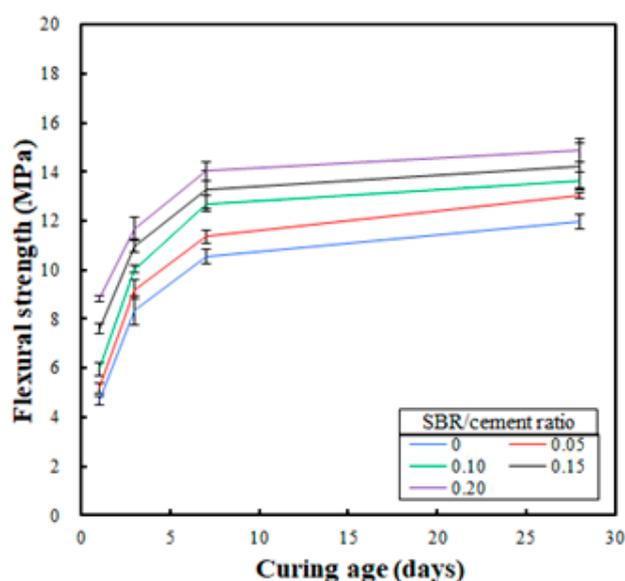
**Figure 11.** Comparison of printed specimens' flexural strength test results for different SBR/cement ratios.
