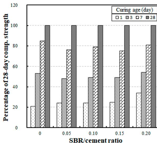
**Figure 4.** Relative gains in compressive strength and SBR/cement ratios for cast specimens with different curing ages.
