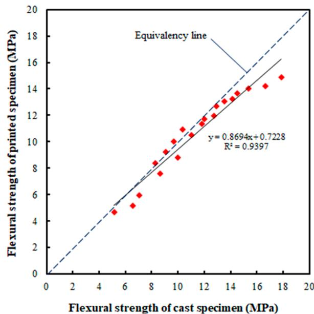
Figure 13. Relationship between cast and printed specimens' flexural strengths.
