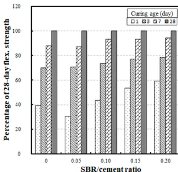
**Figure 12.** Relative gains in flexural strength and SBR/cement ratios for printed specimens with different curing ages.
