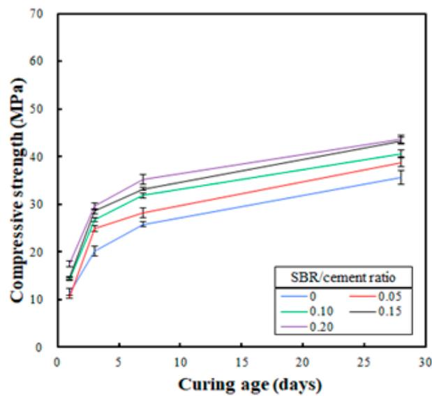
**Figure 5.** Comparison of printed specimens' compressive strength test results for different SBR/cement ratios.
