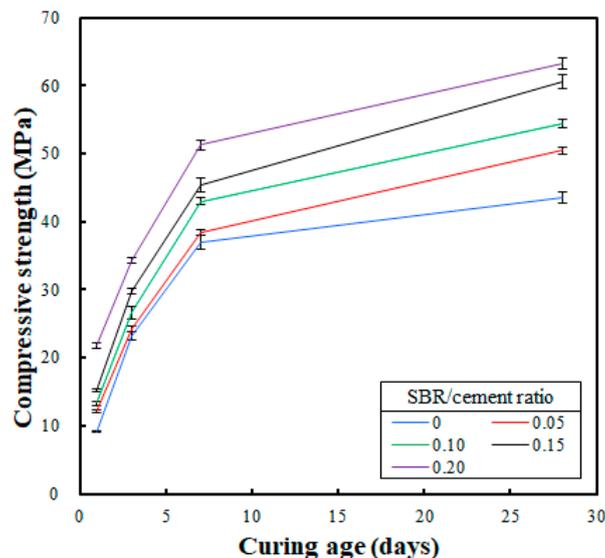
**Figure 3.** Comparison of cast specimens' compressive strength test results for different SBR/cement ratios.
