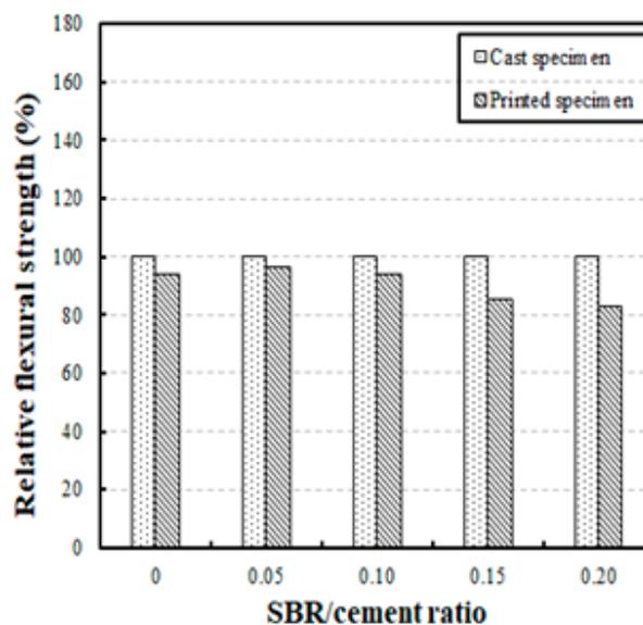
Figure 14. Relative flexural strengths for the cast and printed specimens.
