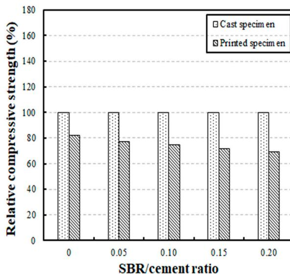
Figure 8. Relative compressive strengths of the cast and printed specimens.
