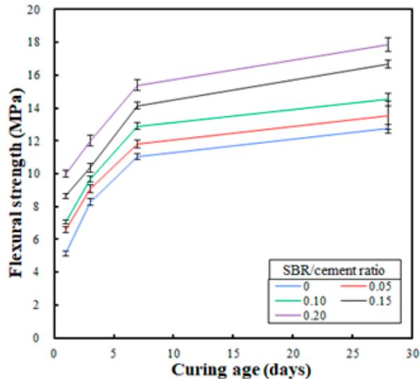
Figure 9. Comparison of cast specimens’ flexural strength test results for different SBR/cement ratios.
