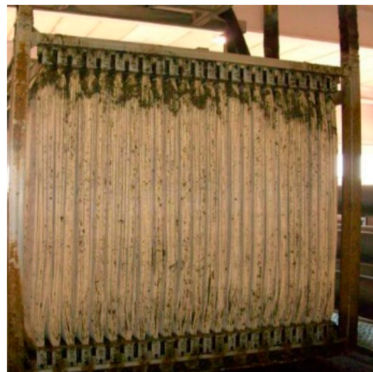
Figure 7. Membrane cassette with aeration and permeation ducts.
