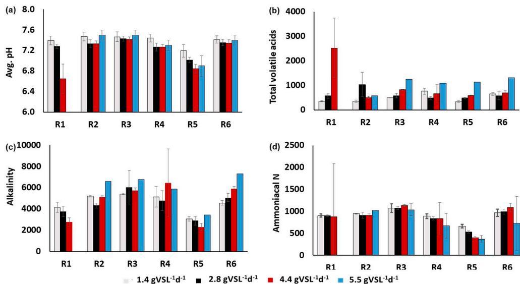
**Figure 1.** Average observed values of (a) pH; (b) total volatile acids [ $\text{mgCH}_3\text{COOH L}^{-1}$ ]; (c) alkalinity [ $\text{mg CaCO}_3\text{ L}^{-1}$ ]; (d) ammoniacal nitrogen [ $\text{mg NH}_3\text{-N L}^{-1}$ ]. Co-substrates: R1—none; R2—AW (acid whey); R3—ED (energy drinks); R4—WB (wasted bread); R5—PN (paper napkins); R6—CM (cow manure).
