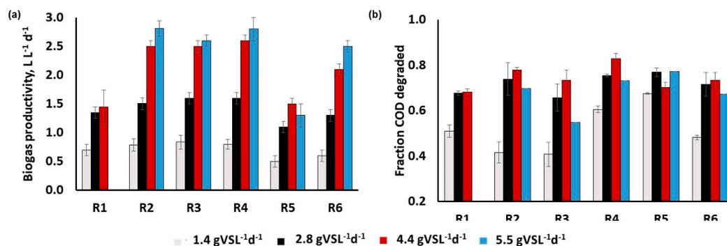
**Figure 4.** Parameters indicative of process efficiency: (a) biogas productivity expressed as the volume of biogas produced per unit volume of the reactor per day; (b) average fractional COD (chemical oxygen demand) degradation at each OLR (organic loading rate). Co-substrates: R1—none; R2—AW (acid whey); R3—ED (energy drinks); R4—WB (wasted bread); R5—PN (paper napkins); R6—CM (cow manure).
