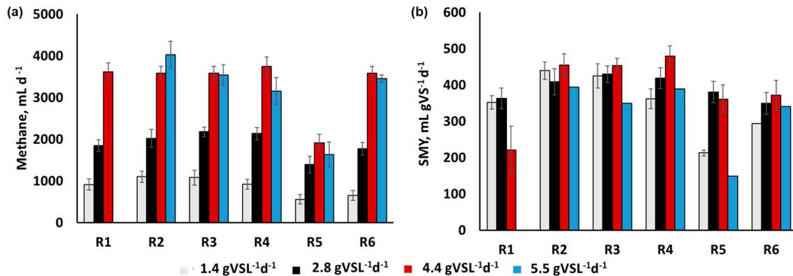
**Figure 3.** (a) Daily average methane production rate [ $\text{mL d}^{-1}$ ]; (b) Specific methane yield (SMY) [ $\text{mL gVSL}^{-1}\text{d}^{-1}$ ]. Co-substrates: R1—none; R2—AW (acid whey); R3—ED (energy drinks); R4—WB (wasted bread); R5—PN (paper napkins); R6—CM (cow manure).
