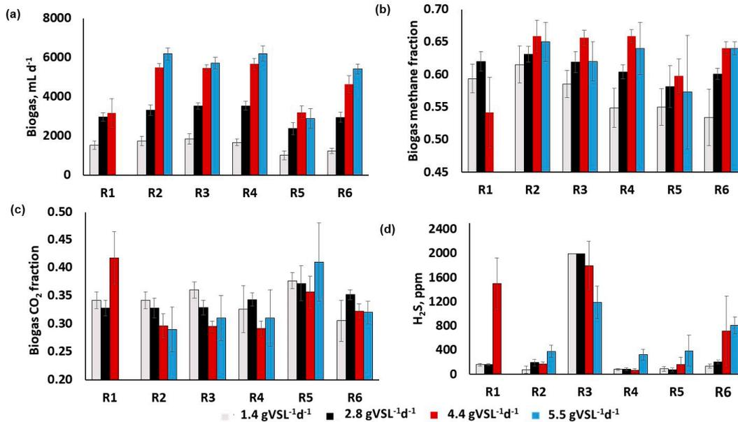
**Figure 2.** Biogas properties: (a) average daily biogas production rate; (b) methane fraction; (c) CO<sub>2</sub> fraction; (d) H<sub>2</sub>S concentration [ppm]. Co-substrates: R1—none; R2—AW (acid whey); R3—ED (energy drinks); R4—WB (wasted bread); R5—PN (paper napkins); R6—CM (cow manure). For R3, the H<sub>2</sub>S concentration reached a detection limit of 2000 ppm of the instrument.
