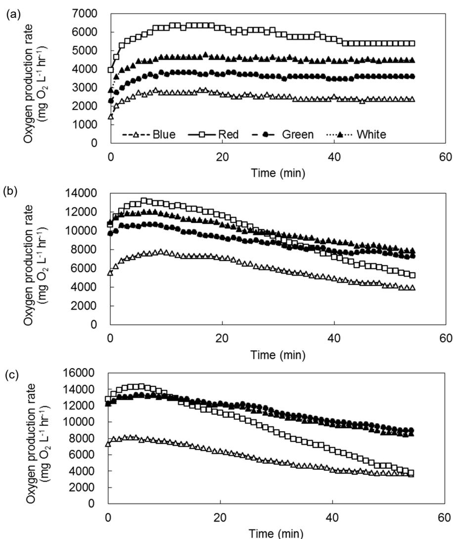
**Figure 6.** The oxygen production rate at a high microalgal–bacterial consortia concentration, where the light intensity is (a) 1000, (b) 2000, and (c)  $3000 \mu\text{mol m}^{-2} \text{s}^{-1}$ .
