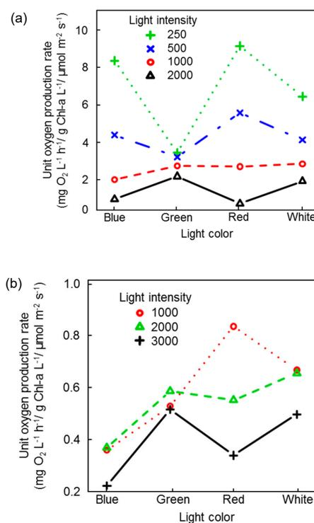
**Figure 9.** Interaction between light intensity ( $\mu\text{mol m}^{-2} \text{s}^{-1}$ ) and color. (a) Low microalgal–bacterial consortia concentrations and (b) high microalgal–bacterial consortia concentrations.
