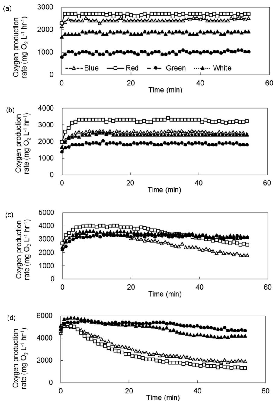
**Figure 5.** The oxygen production rate at low concentration of the microalgal–bacterial consortia where the light intensity is (a) 250, (b) 500, (c) 1000, and (d)  $2000 \mu\text{mol m}^{-2} \text{s}^{-1}$ .
