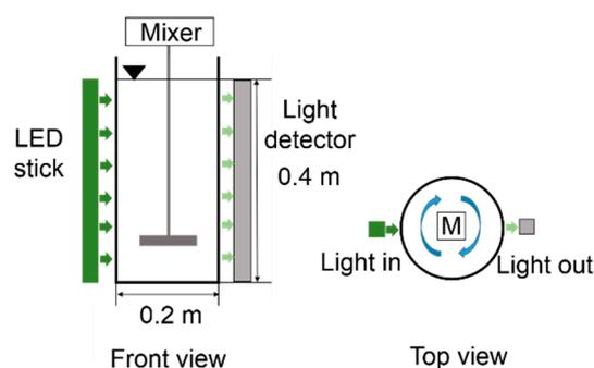
**Figure 3.** Schematic diagram of a batch reactor for inhibition of photosynthetic activities.
