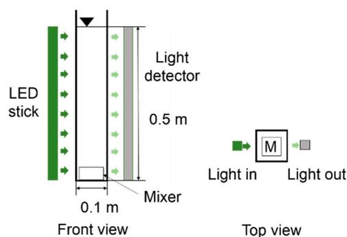
**Figure 2.** Schematic diagram of a rectangular reactor for light transmittance study.
