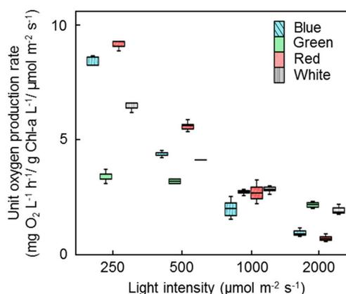
**Figure 7.** The average oxygen production rate at low microalgal–bacterial consortia concentrations during the 54 min illumination period.
