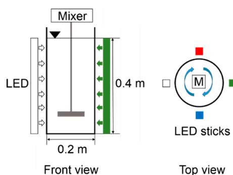
**Figure 1.** Schematic diagram of a batch reactor for cultivation of microalgal–bacterial consortia.
