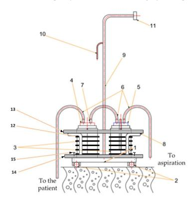
**Figure 4.** The constructive scheme of the complete and reusable pleural drainage system: 1—supporting plate; 2—legs; 3—graduated glass containers; 4—silicone covers; 5—centering prism; 6—tube connections; 7—communication channels; 8—supporting wires; 9—rod; 10—hook; 11—handle; 12—rubber protection ring; 13—upper protection plate; 14—lower protection plate; 15—fixing screw.
