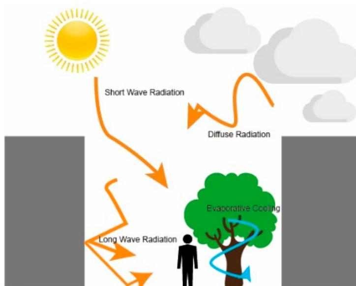
**Figure 1.** Outdoor energy exchange between the street and outdoor environment.
