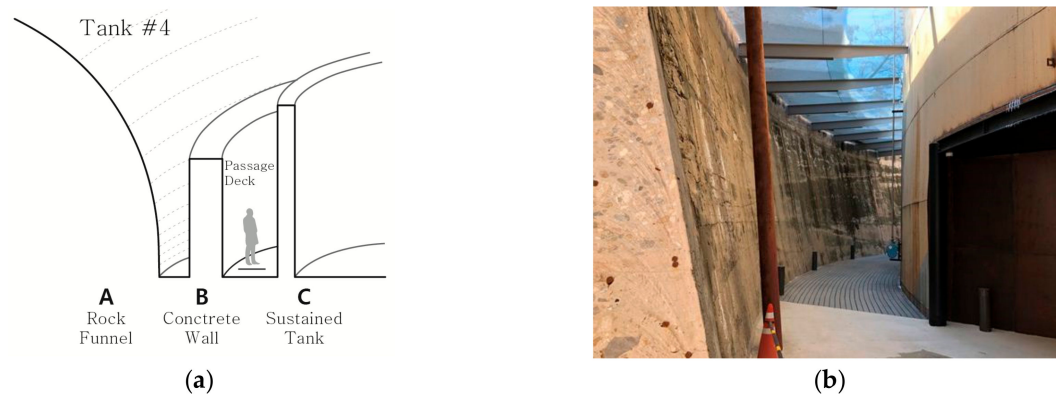
Figure 9. Features of Tank 4, (a) combination of elements, (b) internal space with glass walls and a roof (Credit: Authors).
