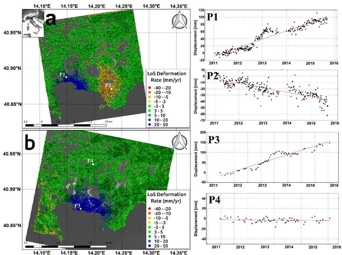
**Figure 5.** Campi Flegrei 2011–2015 uplift highlighted by COSMO-SkyMed interferometric synthetic aperture radar (InSAR) data. Deformation trend estimated along the ascending (a) and descending (b) orbits. In the right panels, the time series of four points are shown.
