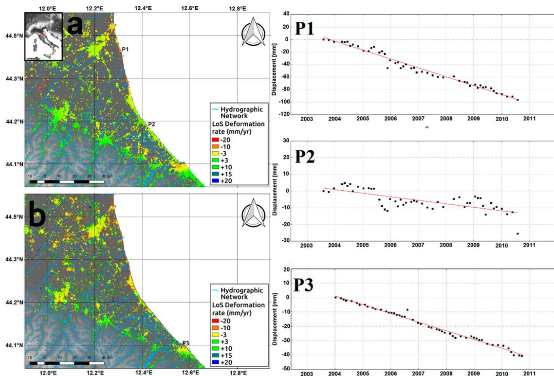
**Figure 3.** Deformation trend of Ravenna coastal area retrieved by ascending (a) and descending (b) ENVISAT data. On the right panels, the time series extracted by three points on the two maps are shown.
