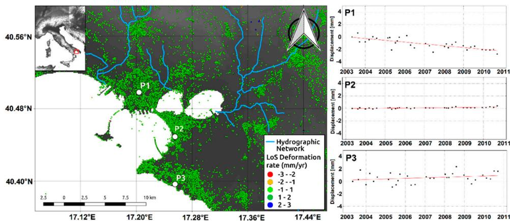
Figure 8. InSAR analysis revealing general stability in the Taranto gulf with very slight subsidence detected only in the northern part of the city (P1 point).
