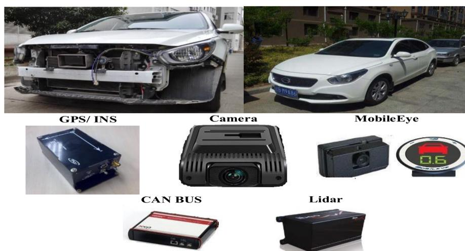
**Figure 3.** Experimental vehicle and equipment.
