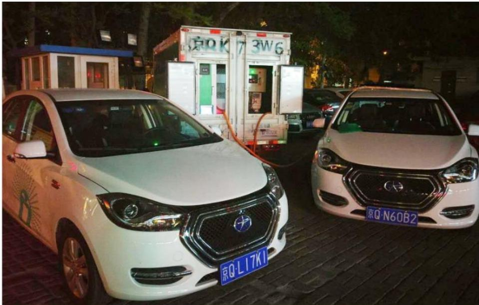
**Figure A3.** The mobile charging car is providing charging service for two vehicles at the same time.
