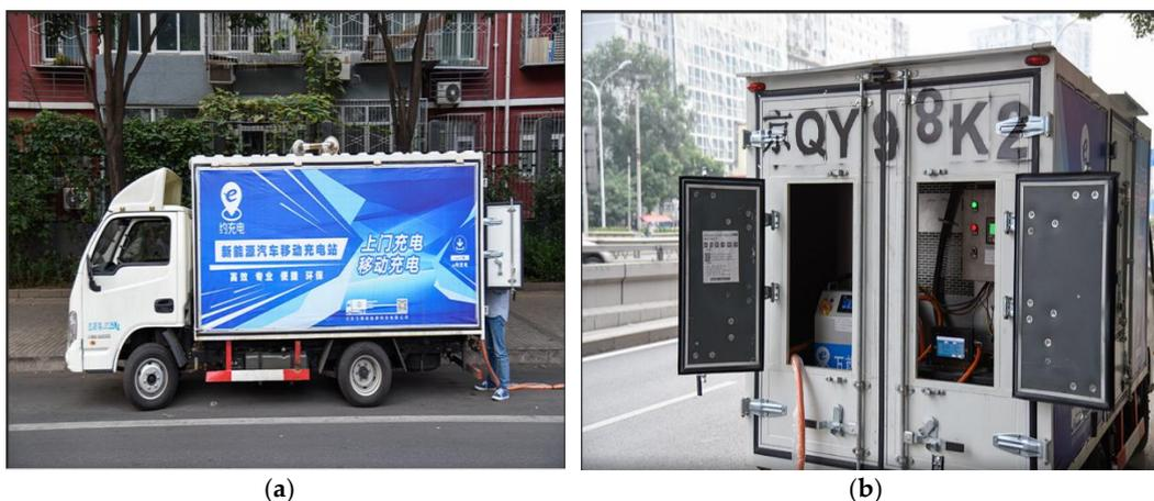
**Figure A2.** The mobile charging vehicle and charging equipment. (a) The mobile charging vehicle; (b) The charging equipment of the car.
