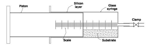
**Figure 2.** Glass syringe to determine the bio-methane potential in HBT anaerobic batch assay (adapted from Mittweg, et al. [29]).
