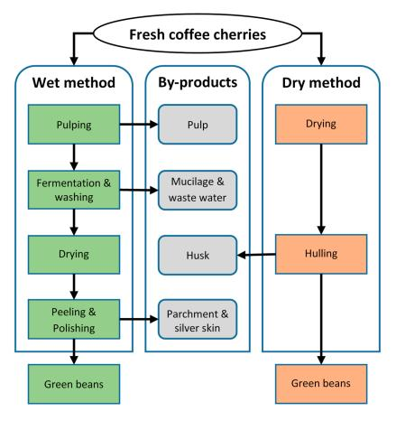
Figure 1. Primary coffee processing pathways to produce green beans following the dry and wet method.
