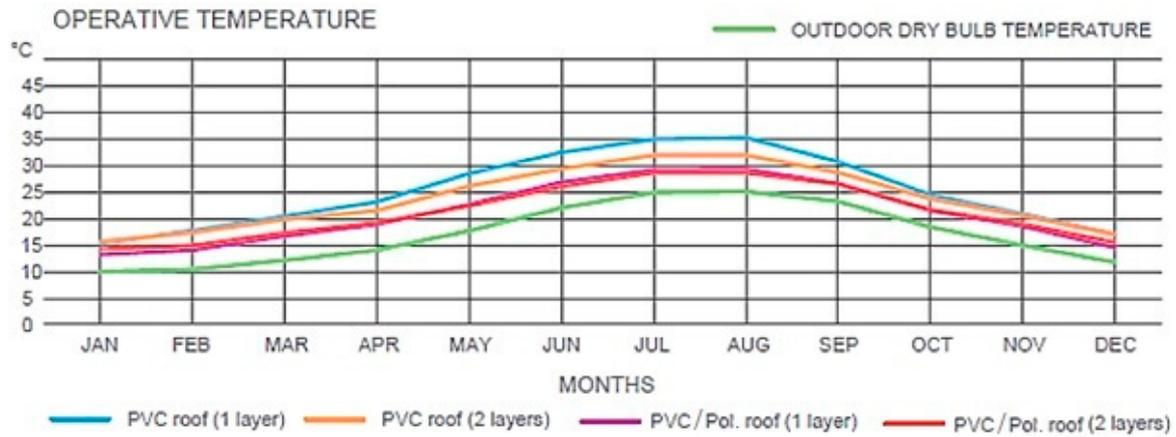
**Figure 12.** Case 2: monthly average of the operative temperature for the four envelope configurations analysed.
