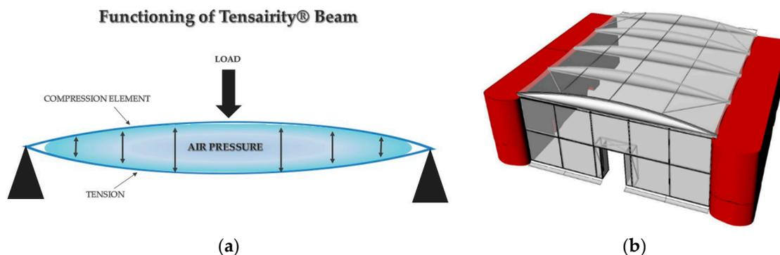
**Figure 4.** Tensairity® Beam: (a) The functioning scheme of a pneumatic beam [41–43]; (b) Example of Tensairity® beams mounted on semitrailers.
