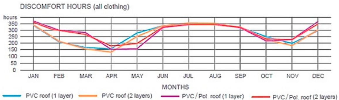
**Figure 13.** Case 2: monthly average of the Discomfort Hours for the four envelope configurations analysed.
