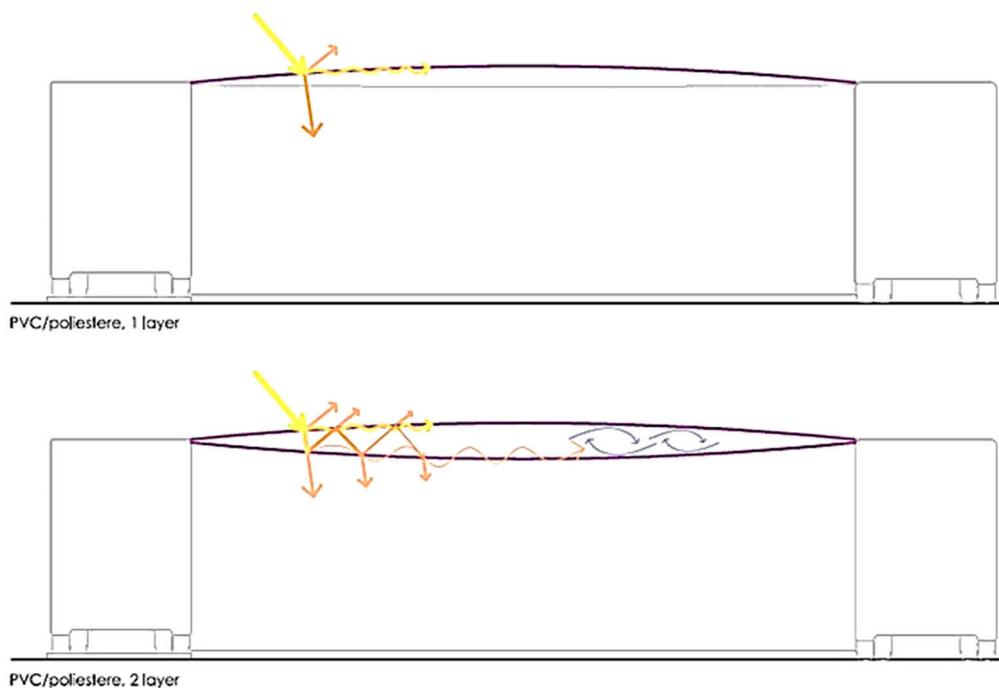
**Figure 9.** Diagram showing heat transmission modes in the coverage configurations analysed: orange lines relate to solar transmission toward the membrane, blue lines represent the steady air gap.
