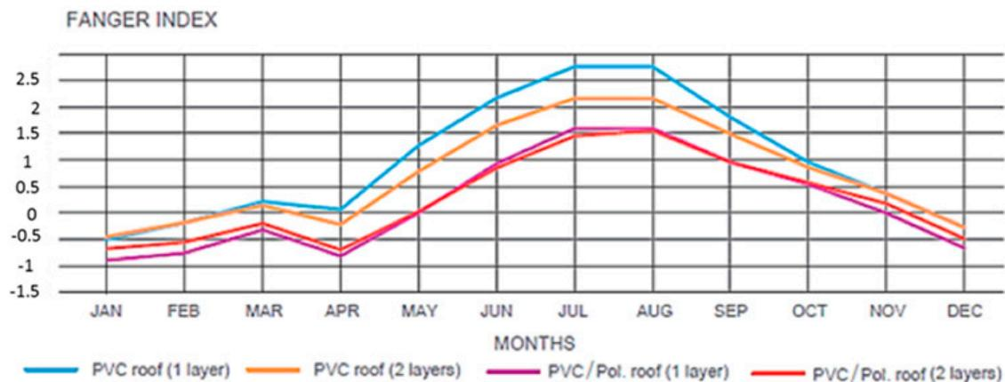
**Figure 14.** Case 2: monthly average of the Fanger Index for the four envelope configurations analysed.
