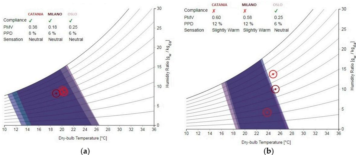
Figure 8. Psychrometric chart of Ducati Pavilion based on one layer of PVC and operative HVAC system: (a) January behaviour; (b) July behaviour (charts produced using CBE Thermal Comfort Tool).
