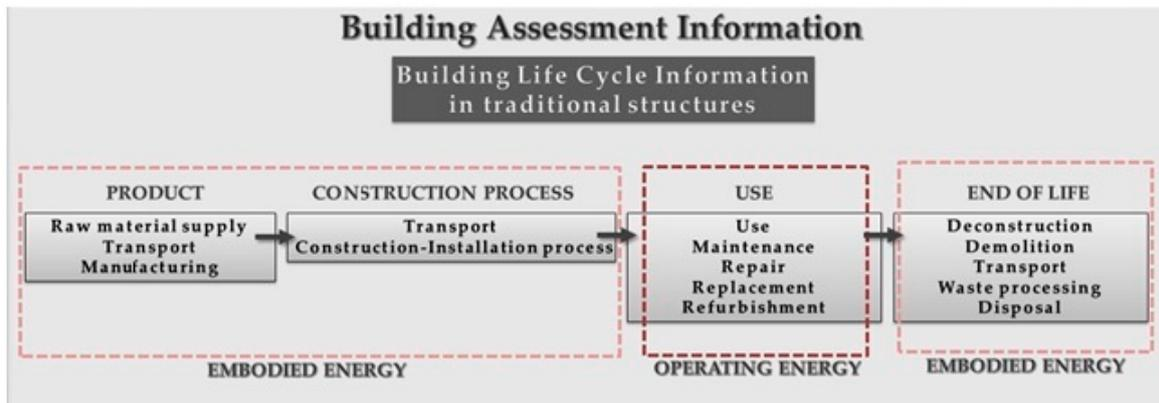
Figure 1. The life cycle of traditional structures.
