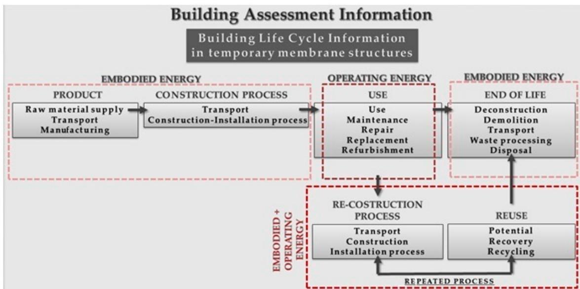
Figure 2. The life cycle of temporary membrane structures.
