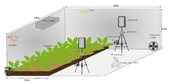
Figure 2. Schematic drawing of the test room to evaluate the PM deposition of GR and LW species.
