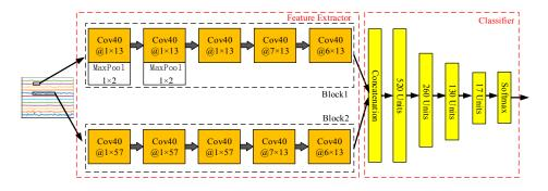
Figure 2. Schematic of C-B1PB2 used on the sEMG signals.
