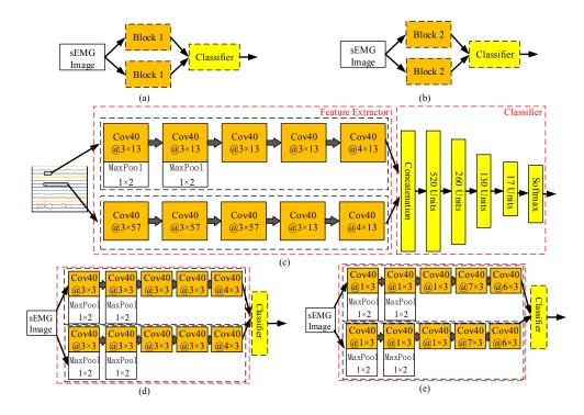
**Figure 3.** Schematics of three reference experiments: (**a**) convolution with two parallel Block 1 (C-2B1); (**b**) convolution with two parallel Block 2 (C-2B2); (**c**) convolution with a different kernel (C-DK); (**d**) convolution with the small kernel(C-SK); and (**e**) convolution with the small kernel 2 (C-SK2).
