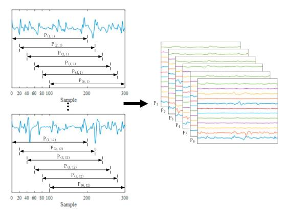
**Figure 1.** Converting the sEMG signals to sEMG images by sliding window.  $P_{(a,b)}$  represents a segment of sEMG signal from electrode *b* at the time *a*.  $P_a$  represents the sEMG signals from 12 electrodes at the time *a*.
