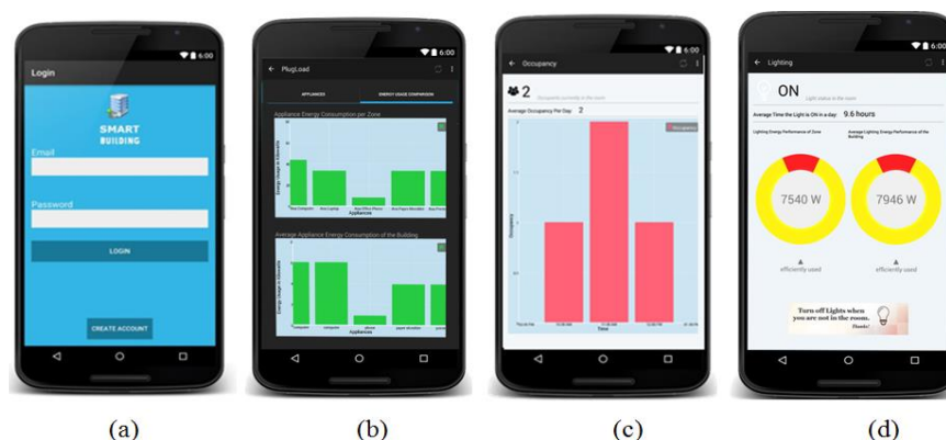
Figure 7. Building Brain features: (a) secure login; (b) energy Consumption of plug load; (c) number of occupancy; and (d) lighting information.
