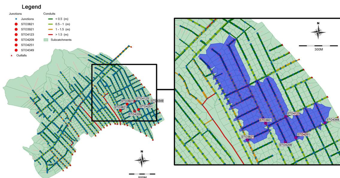
**Figure 4.** Deployed detention ponds with their dedicated drainage area (location: 26°18' S, 48°49' W).
