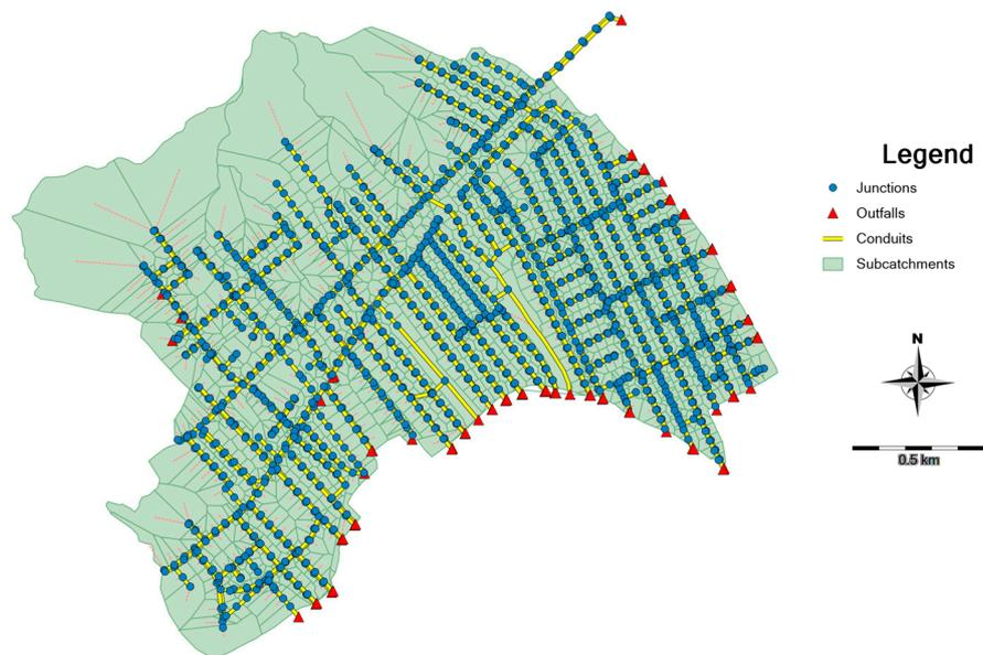
**Figure 2.** Representation of the storm drain system in the PCSWMM model (location:  $26^{\circ}18' S$ ,  $48^{\circ}49' W$ ).
