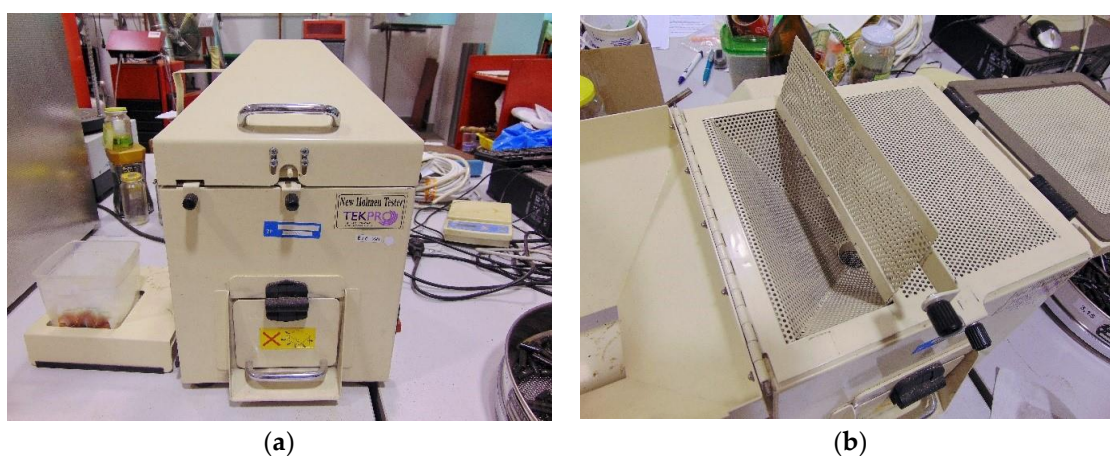
Figure 6. The New Holmen Tester pellet durability tester: (a) outside of testing device, (b) abrasion chamber.
