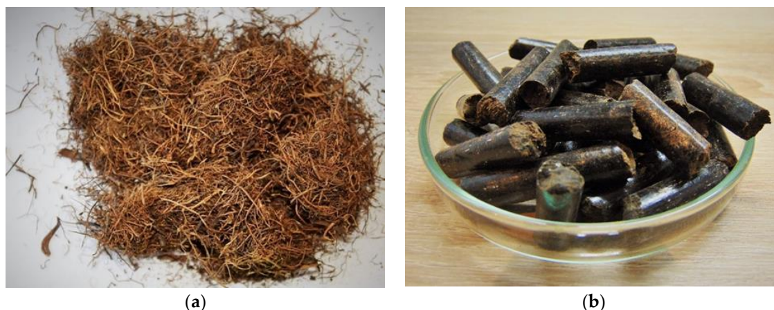
Figure 3. Investigated oil palm EFB: (a) In raw form; (b) in bio-pellet fuel form.
