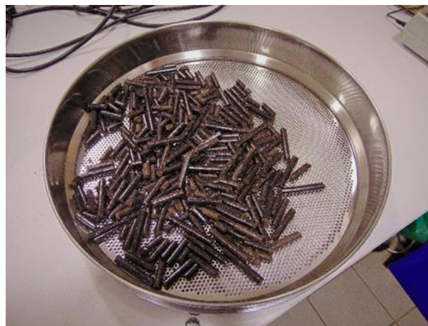
Figure 4. Metal sieve used to determine amount of fines produced ( F (%)) with 3.15 mm-diameter round holes.
