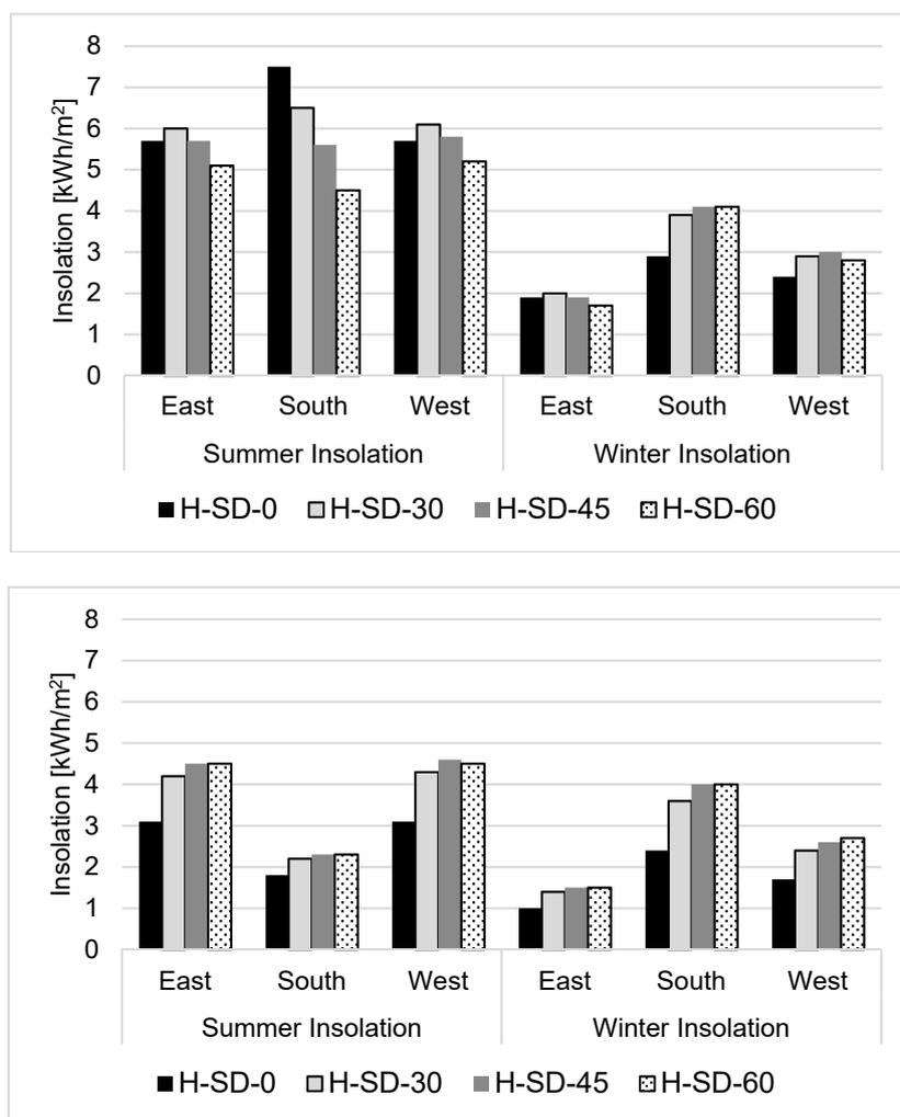
**Figure 3.** Normalised average daily total insolation levels recorded for the different cases of the examined horizontal shading devices at top floor (**top**) and typical floor (**bottom**).
