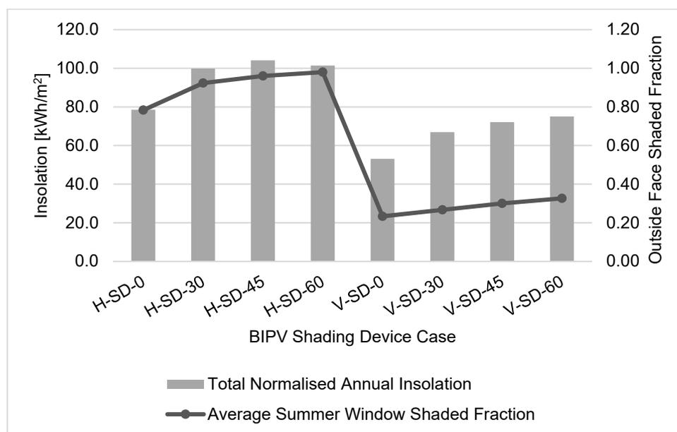
**Figure 6.** Total performance indicators of the examined cases of BIPV shading devices.
