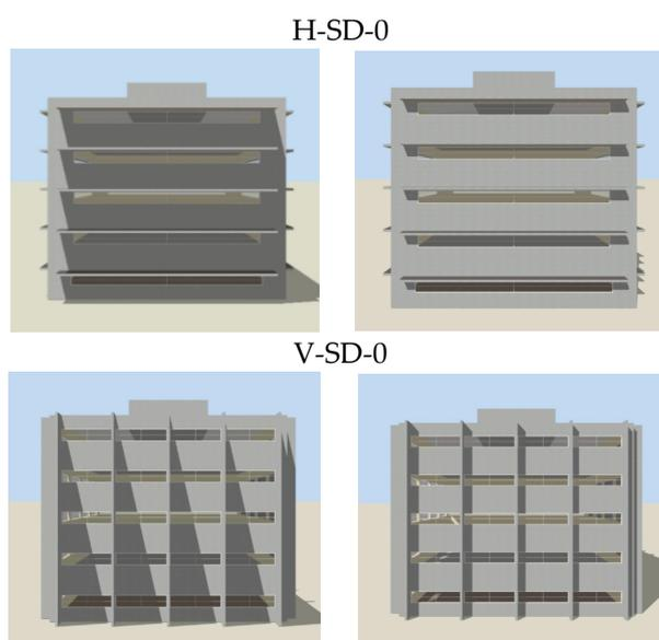
**Figure 4.** Shading patterns observed in cases H-SD-0 and V-SD-0 in summer (left) and winter (right) on the southern facade at 1:00 pm.
