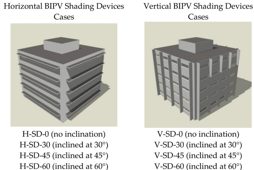
**Figure 2.** The proposed horizontal modelling cases (H-SD) and vertical ones (V-SD), where four BIPV inclination settings are examined.
