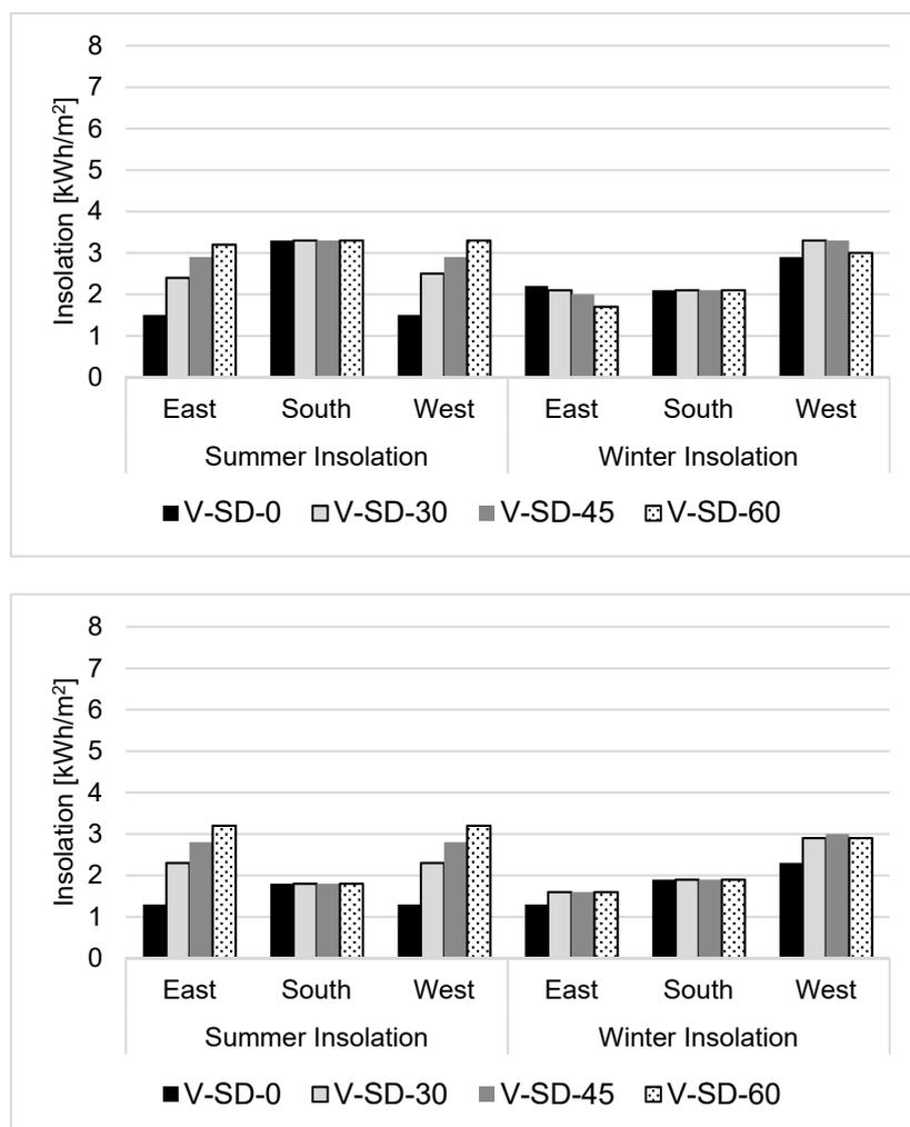
**Figure 5.** Normalised average daily total insolation levels recorded for the different cases of the examined vertical shading devices at the beginning (**top**) and middle (**bottom**) of the building facade.
