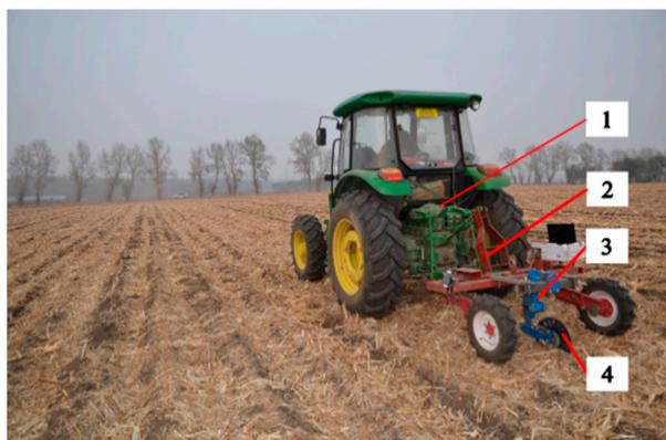
**Figure 2.** Field test site. (1) JOHN DEERE 50PS type tractor, (2) Hanger, (3) Sliding shank, (4) Tested coulters.
