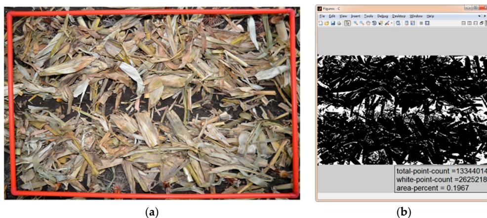
**Figure 4.** Residue coverage measurements: (a) A soil surface image confined by a 1  $\times$  0.65 m quadrat after tillage, (c) A processed image.
