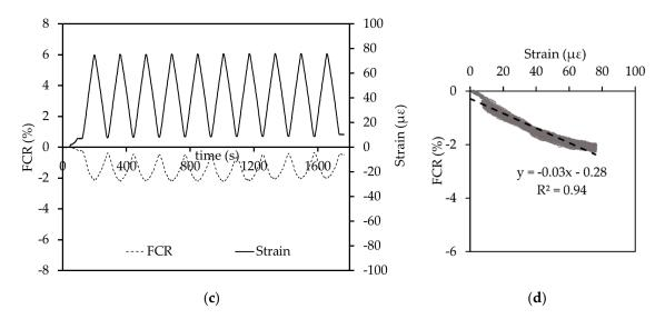
**Figure 7.** FCR and strain vs. time of the (a) dried 0.2VCF specimen and (b) dried GNP-0.2RCF specimen under cyclic loading. FCR-strain trend line of the (c) dried 0.2VCF specimen and (d) dried GNP-0.2RCF specimen.
