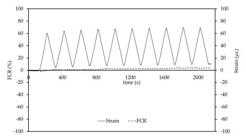
**Figure 6.** FCR and strain vs. time of the 28-day cured GNP-0.2RCF specimen under cyclic loading just after the extraction from the climatic chamber.
