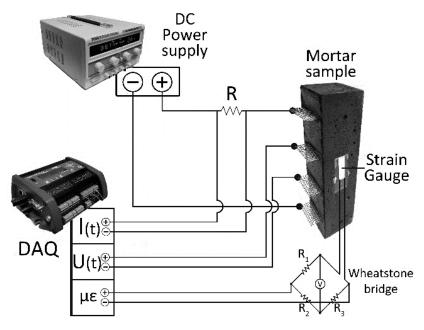
Figure 2. Setup for electrical measurements.
