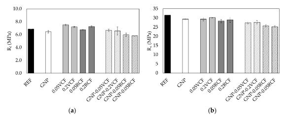
Figure 3. Flexural strength (a) and compressive strength (b) of mortars after 28 days of curing.
