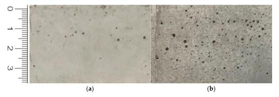
Figure 4. Visual aspect of (a) REF and (b) GNP mortars after 28 days of curing.
