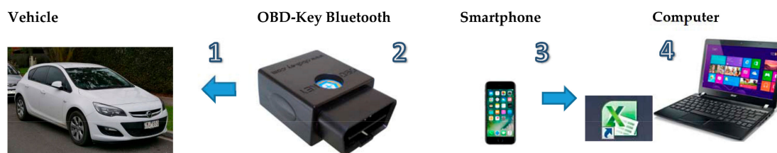
Figure 2. Experimental car data collection through the OBD-key device [38].
