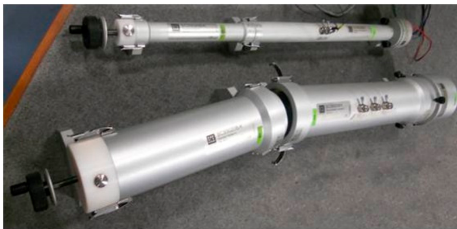
Figure 3. Impedance tubes device used in the experiment to evaluate the acoustic properties of SSFC and WCC in the high frequency range (1000–5000 Hz) and in the low frequency range (100–1200 Hz).
