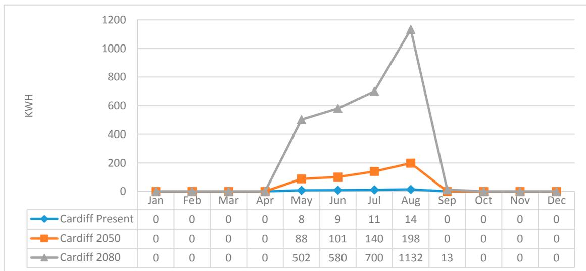
Figure 8. Cooling loads in the current, 2050, and 2080 time slices.
