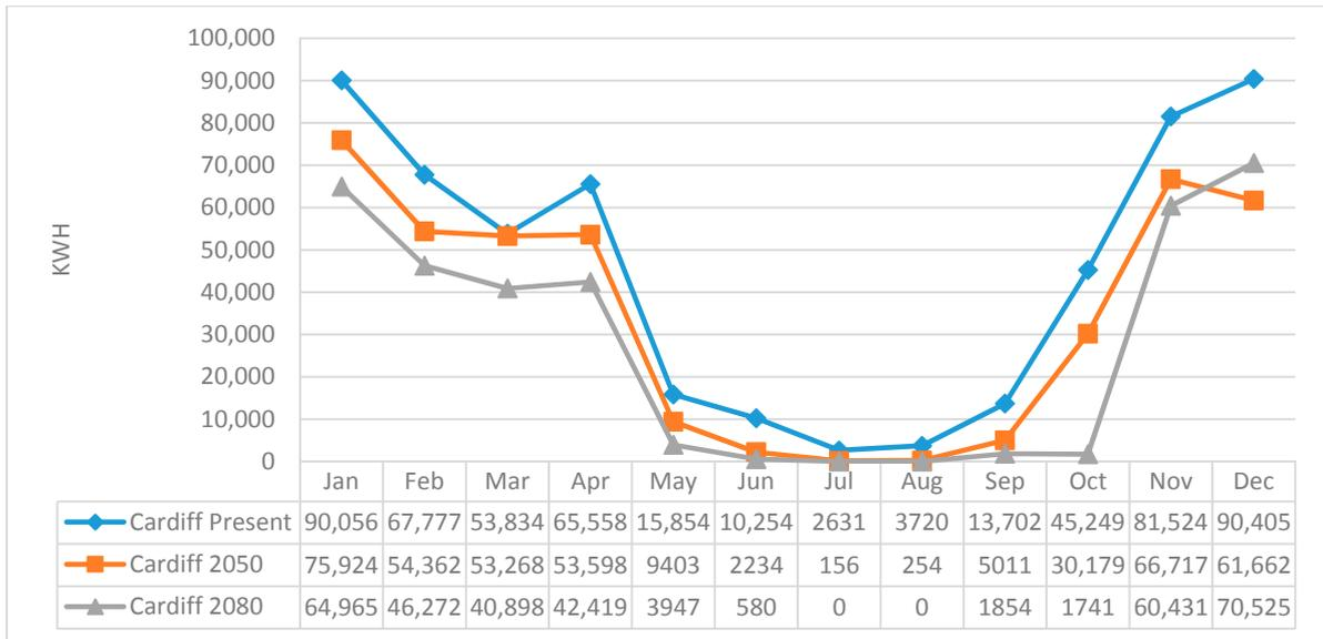
Figure 7. Heating loads in the current, 2050, and 2080 time frames.
