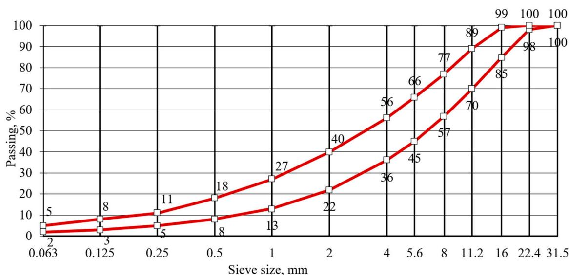
Figure 1. Aggregate gradation limits for double Otta Seal.
