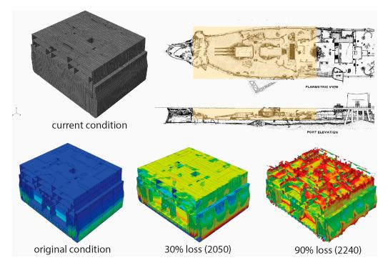
Figure 14. Computer model of the USS Arizona with projected decay of structure. Source: [62].
