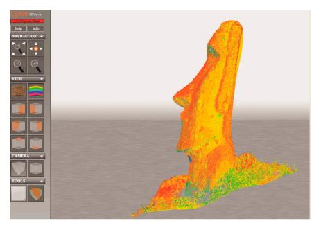
Figure 13. Tripod-mounted terrestrial 3D laser scan of *moai*. Source: CyArk.
