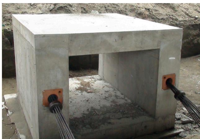
Figure 6. Full-scale pier segment.
