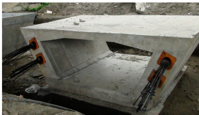
Figure 8. Full-scale box girder segment.
