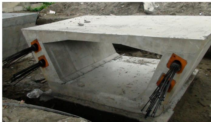
Figure 8. Full-scale box girder segment.
