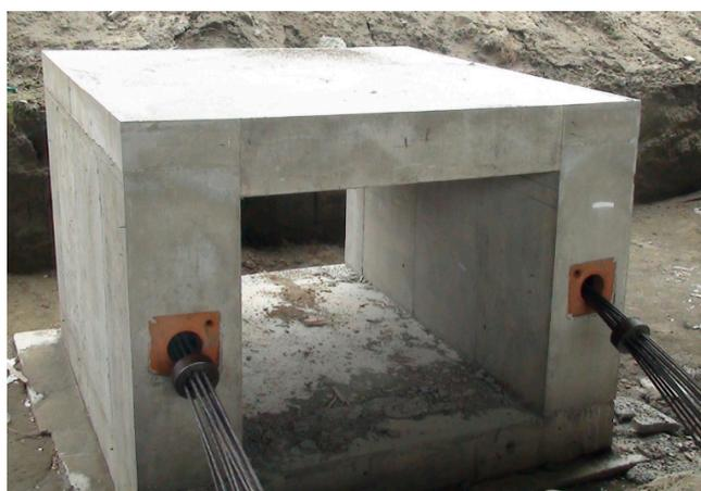
Figure 6. Full-scale pier segment.
