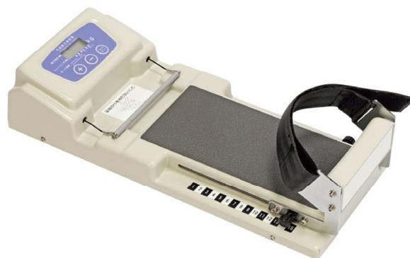
**Figure 2.** Toe grip dynamometer.
