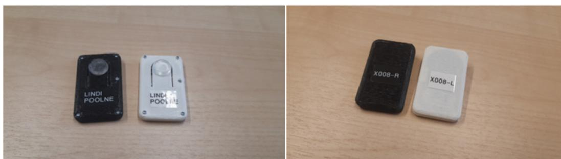
**Figure 2.** Frontal- and back-view of force pressure sensor.
