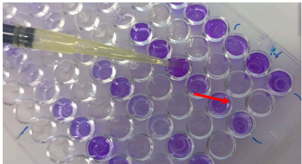
Figure 3. Biofilm formation assay on polyvinyl chloride (PVC) coupons placed in 96-well microplates and stained with crystal violet for biomass quantification. The arrow indicates the position of the PVC coupon placed at the bottom of each well. After incubation with microbial suspensions and treatment with various concentrations of Syzygium aromaticum essential oil, residual biofilm biomass was visualized by 1% crystal violet staining. The intensity of the purple coloration reflects the density of the adherent biofilm on the PVC surface, with lighter wells corresponding to greater antibiofilm activity of the essential oil.
