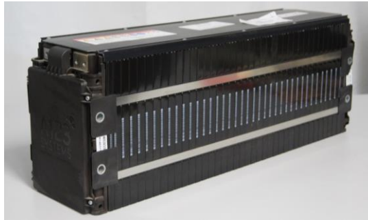
Figure 8: One module with 78 pouch cells [4]
