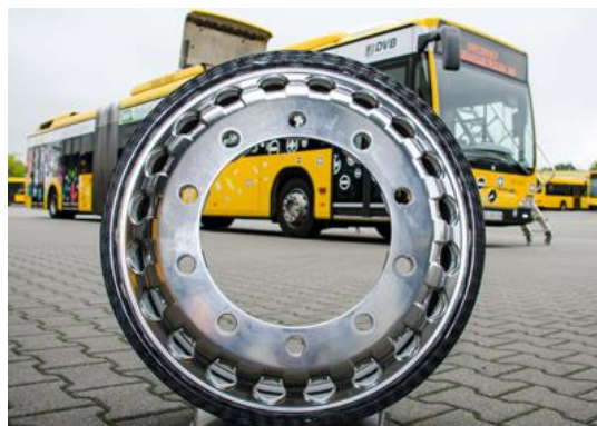
Figure 4: CFRP Light-weight rim [10]
