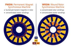
Figure 1: E-machine topologies under study: PMSM (left) and WRSM (right), both having a nominal mechanical power  $P_{nom} = 31$ kW at  $f_{nom} = 400$ Hz.
