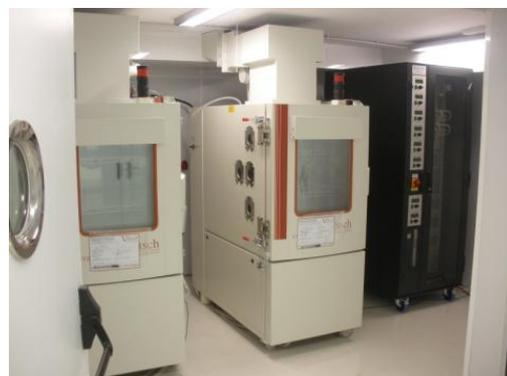
Figure 1: Battery cycler and the climatic chamber.
