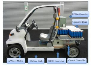
Fig. 2: Hybrid Electric Vehicle Prototype
