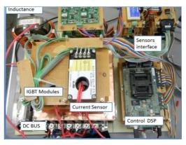
Fig.6. Converter Prototype for SC power interface
