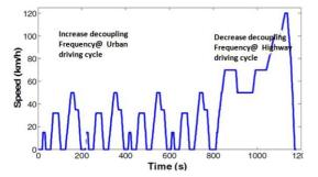
Fig 6 NEDC speed profiles from ref. [6]
