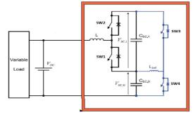
Fig.7 Half controlled converter structure for HCC
