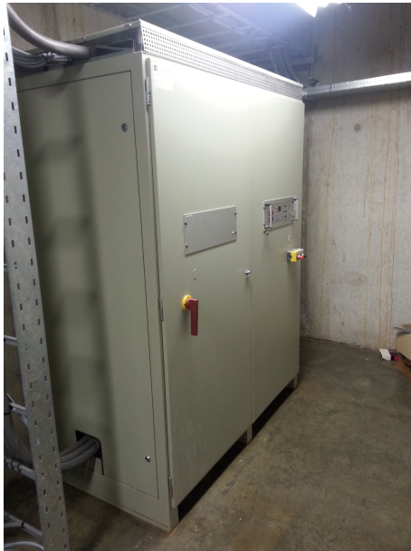
Figure 4: Digatron BS-400 battery test system
