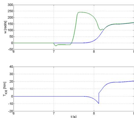
Figure 24: Simulation results of ICE speed, sun shaft speed and ICE torque during ICE starting (No13 in Table 4)
