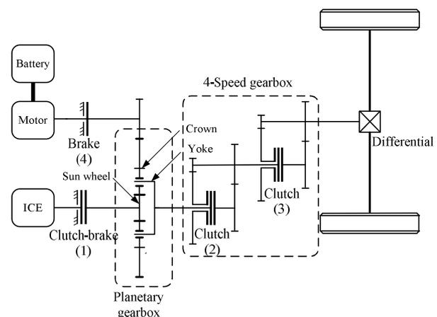
Figure1: Configurations of the improved CHPTD with gearbox
