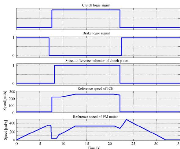
Figure 10: Control signal generated by control logic block
