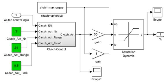
Figure 11: Simulation model of clutch current control unit
