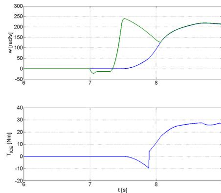
Figure 25: Simulation results of ICE speed, sun shaft speed and ICE torque during ICE starting (No6 in Table 4)
