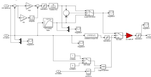
Figure 5: Simulation model of internal combustion engine
