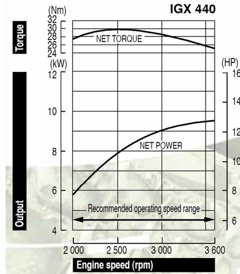
Figure 6: The external characteristic of Honda IGX440 engine
