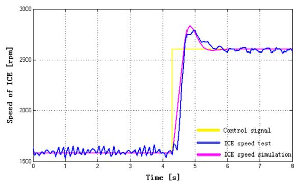
Figure 7: Step response of internal combustion engine
