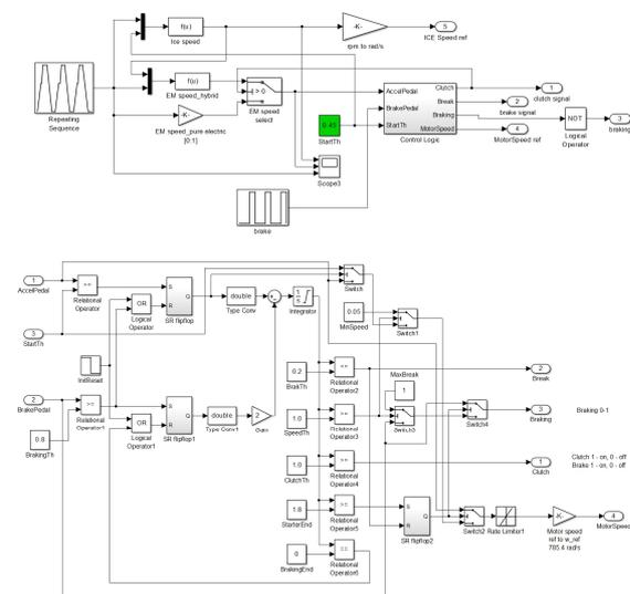
Figure 9: Driving cycle and control logic block
